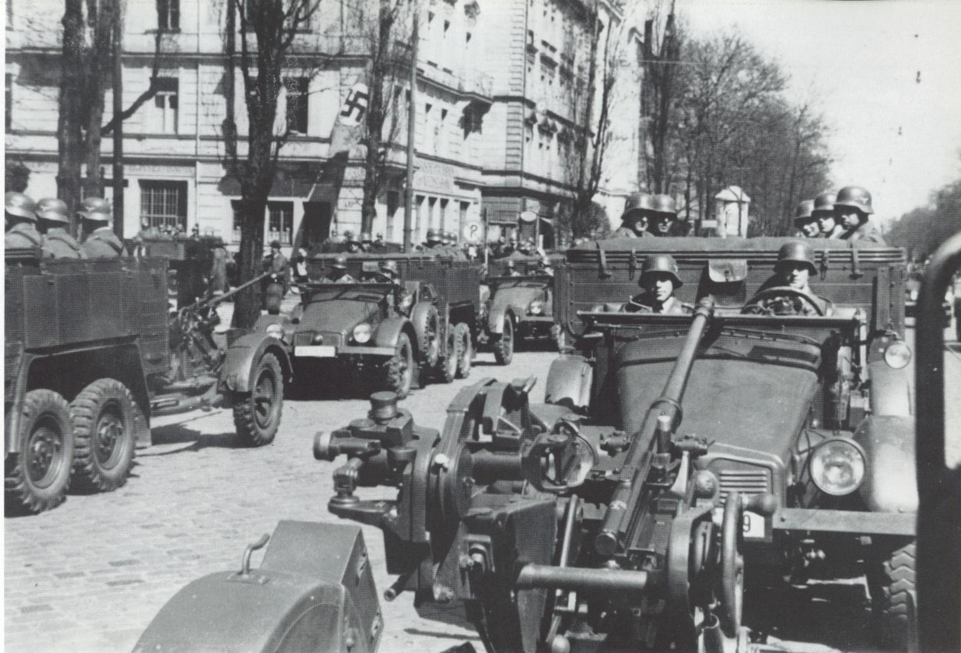
Troop parade in Munich on April 20, 1939. Krupp L 2 H 143 as light anti-aircraft gun truck (Kfz.81) with 20mm Flak 30 on Sd.Ah.51. At that time, Flak Regiment 5 and the 1st Flak Unit 75 (ex-II./5) were located in Munich.
