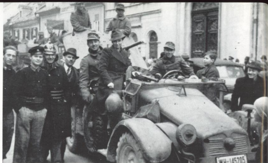
Panzerjäger Unit 44 arrives at Celja on the Save in April of 1941. A Krupp L 2 H 43 with fixed 37mm Pak gun and extended shield. Note the high camouflaged headlights and the MP 28/11 on the windshield.
