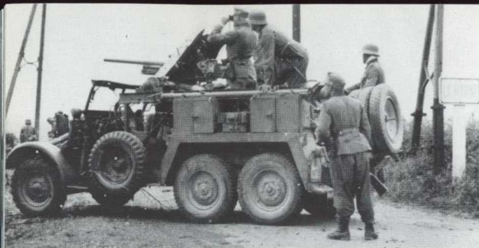
Above: Panzerjäger Unit 44 (1st Mountain Division) had a series of towing trucks with built-in 37mm Pak guns (rebuilt by the troops). Here such an "assault gun" fires across the Marne at Chateau-Thierry on June 12, 1940. Note the pressed-steel frame with the wheel hub lashed to it, the strut on the side and the way the gun wheels are carried. By the short distance between the rear axles, this is a Krupp L 2 H 43.
