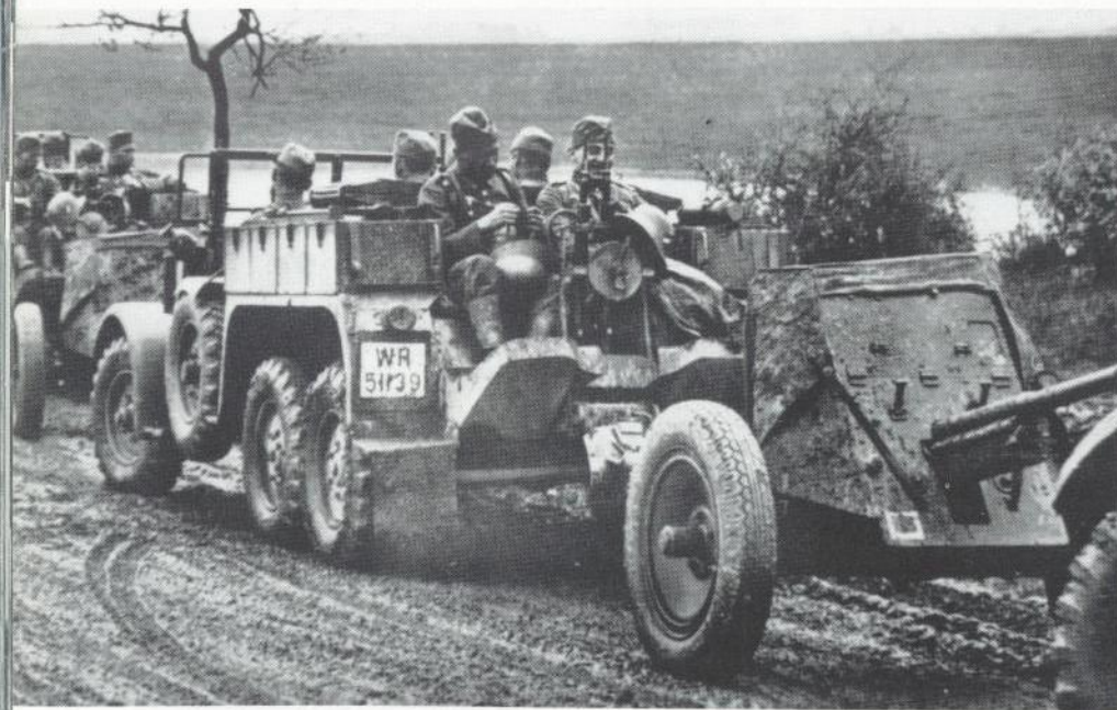
Above: Krupp L 2 H 143 as towing truck (Kfz.69) with 37mm Pak in France, 1940. Here one sees another type of ammunition cases, tall with handles.
