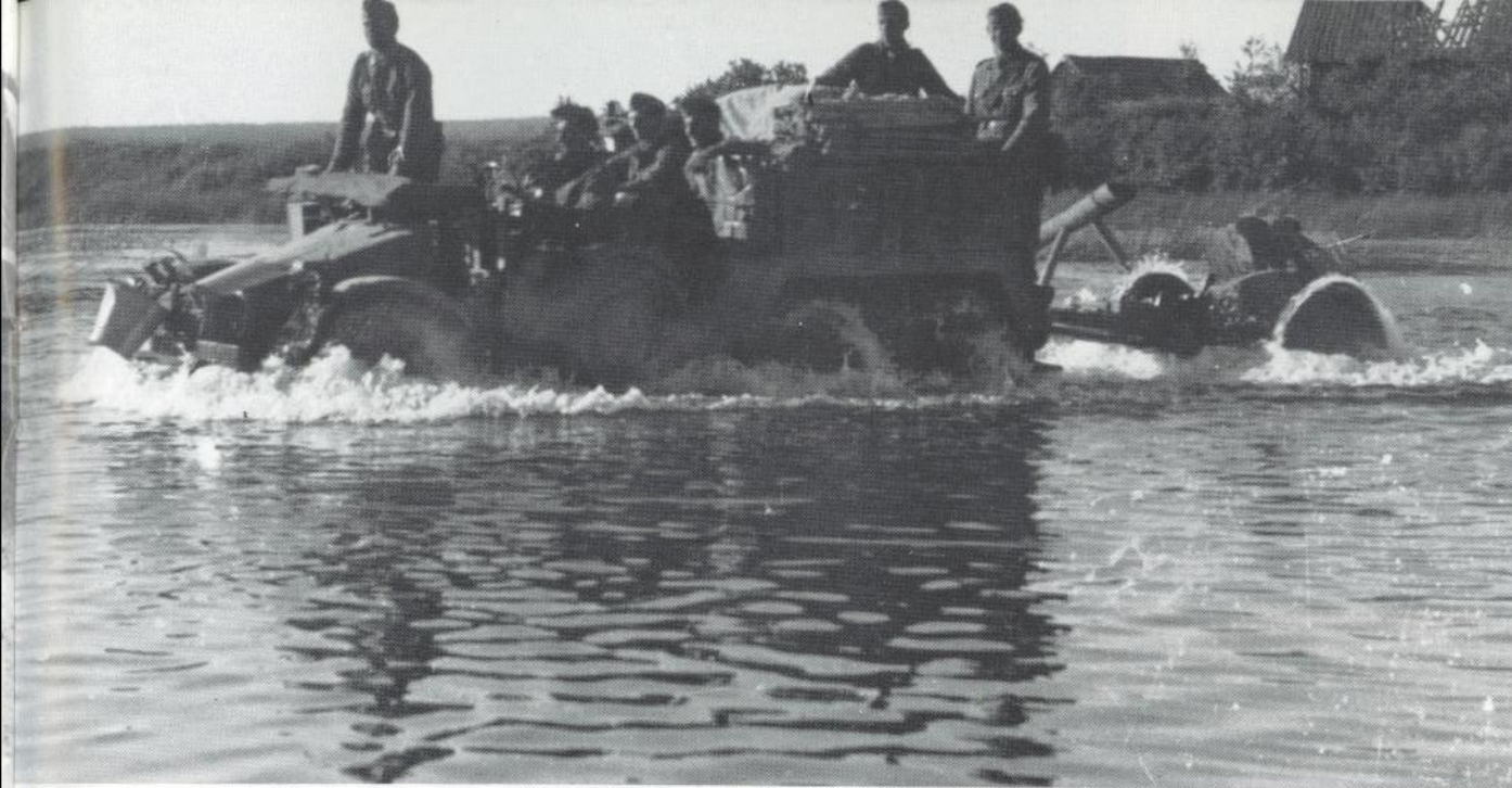
Upper left: Leningrad area, 1941. Krupp L 2 H 143 as towing truck (Kfz.69) with 75mm light infantry gun 18.(BA)
