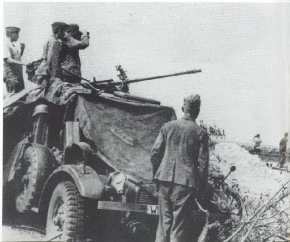
Below: A light anti-aircraft truck (L 2 H 143, Kfz.81) carrying a 20mm Flak 30 gun securing a river crossing. The crew has given themselves a bit of cover by using tent panels.
