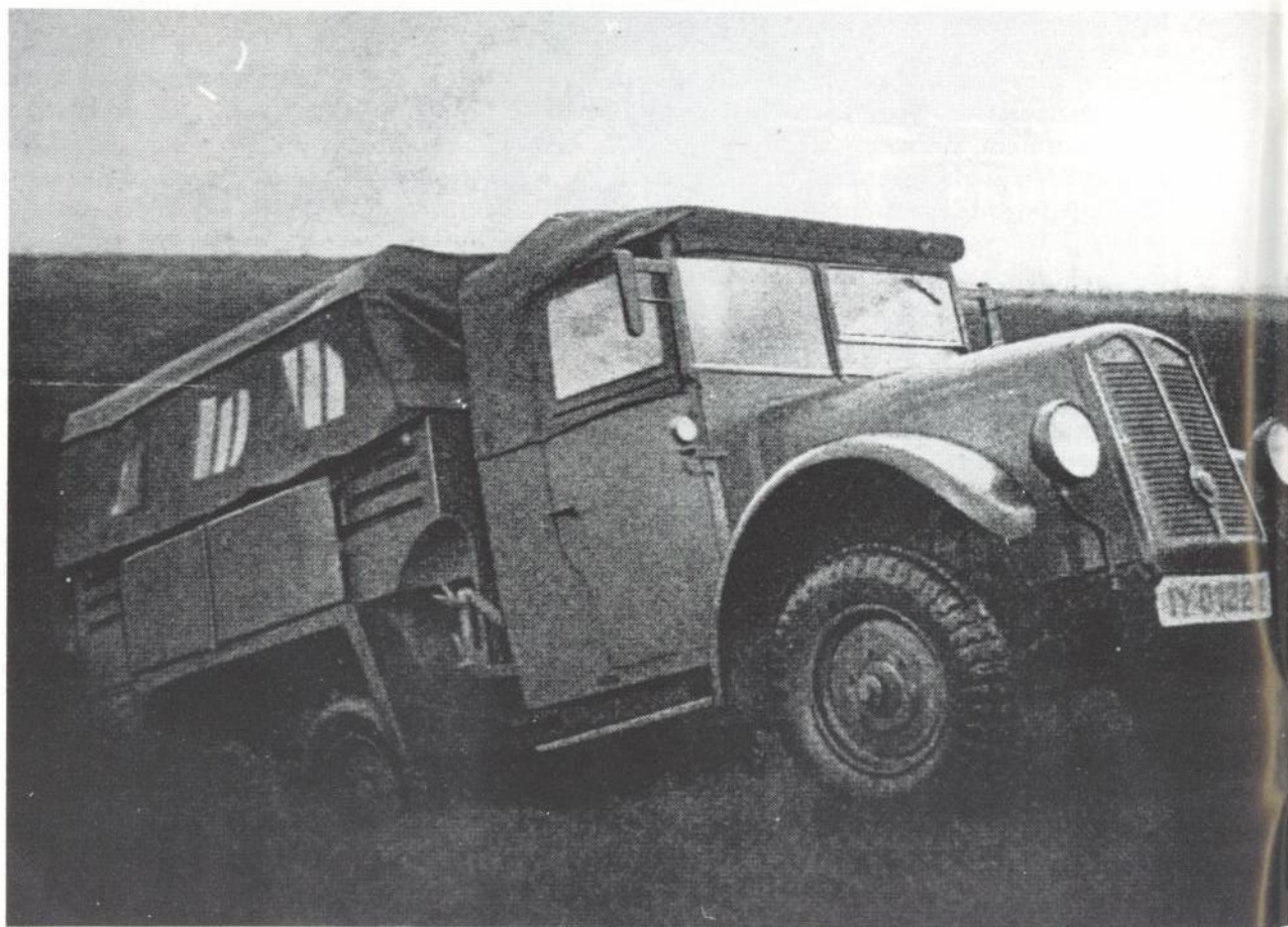
The grandfather of all Krupp army trucks was this 1929 "light off-road truck with air-cooled carbureted or Diesel engine, L 2 H 43 or LD 2 H 43." The engine hood did not yet have the typical angled form, so as to leave room for the bigger (50-HP) Diesel engine. The gasoline engine produced 60 HP.
