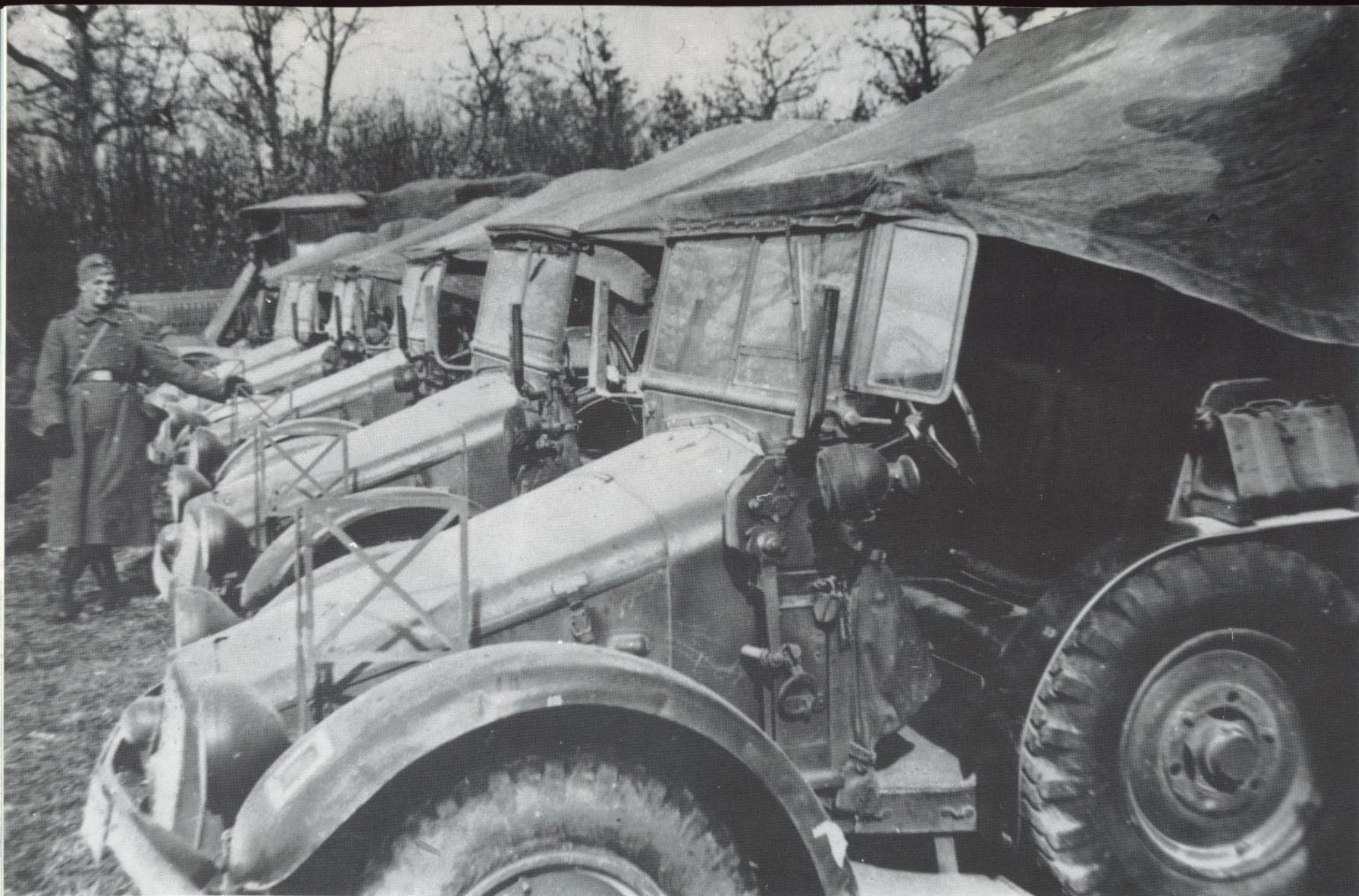
Krupp L 2 H 143 trucks as personnel carriers (Kfz.70) of MG Battalion 6 in Coburg. Note the non-standard technical details of the truck in front: higher cover and spotlight, different attachment of the direction indicators, side wind deflectors, cover snaps and greater distance between windshield and engine hood.
