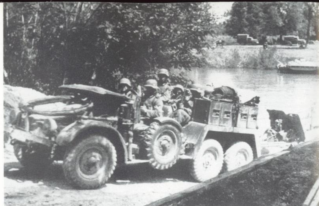
Above: This towing truck (Kfz.69) with 37mm Pak gun has low, wide ammunition cases. The rear spare wheel was apparently removed by the Schirmeister. Note the transverse bridge panels, fire extinguisher at right, and Model 16 helmets.
